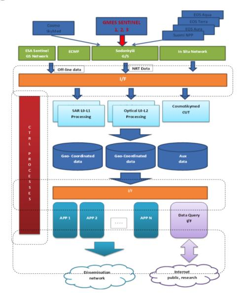
Proposed system structure for service provision including satellite and in situ data acquisition from various sources.
