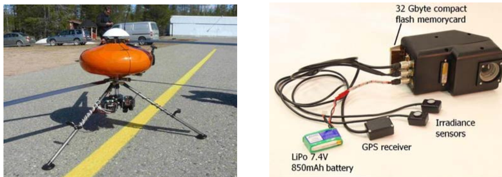
Figure 1. Infotron IT-180 UAV helicopter with both the CIR camera and Hyperspectral imager payload and flight configuration of UASI 2012 hyperspectral Imager.
